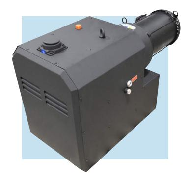
The Airtech VCX positive displacement rotary claw design is air cooled, dry-running and non-contacting. These features, along with quality construction results in a vacuum pump that is extremely high in reliability and a long service life. The non-contact design eliminates internal wear and maintenance. No water levels to check due to air-cooled operation and no sealing or lubricating oil is needed in the pumping chamber.
