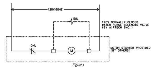
6.6.8 Use of a properly sized magnetic motor starter with heater is required to protect the equipment from electrical failure.
