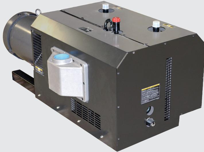
Quality construction and design features make KCP positive displacement rotary claw vacuum pumps extremely reliable and easy to maintain. The KCP's non-contact design reduces internal wear, and air-cooled operation eliminates the need for cooling liquid. The unit is also dry-running, so no sealing or lubrication oil is needed in the pumping chamber.
