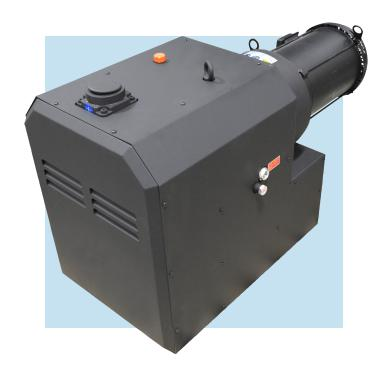
The Airtech PCX positive displacement rotary claw design is air cooled, dry-running and non-contacting. These features, along with quality construction results in a pressure pump that is extremely high in reliability and a long service life. The non-contact design eliminates internal wear and maintenance. No water levels to check due to air-cooled operation and no sealing or lubricating oil is needed in the pumping chamber.
