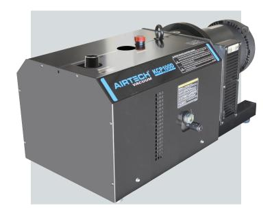
Quality construction and design features make KCP positive displacement rotary claw vacuum pumps extremely reliable and easy to maintain. The KCP's non-contact design reduces internal wear, and air-cooled operation eliminates the need for cooling liquid. The unit is also dry-running, so no sealing or lubricating oil is needed in the pumping chamber.
